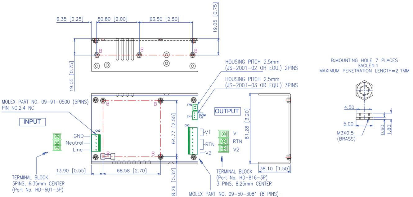
**RL0603DF Series (Enclosed with Top Fan Type): 5(L) x 3.2(W) x 2(H) inches; Weight: 550g.**
