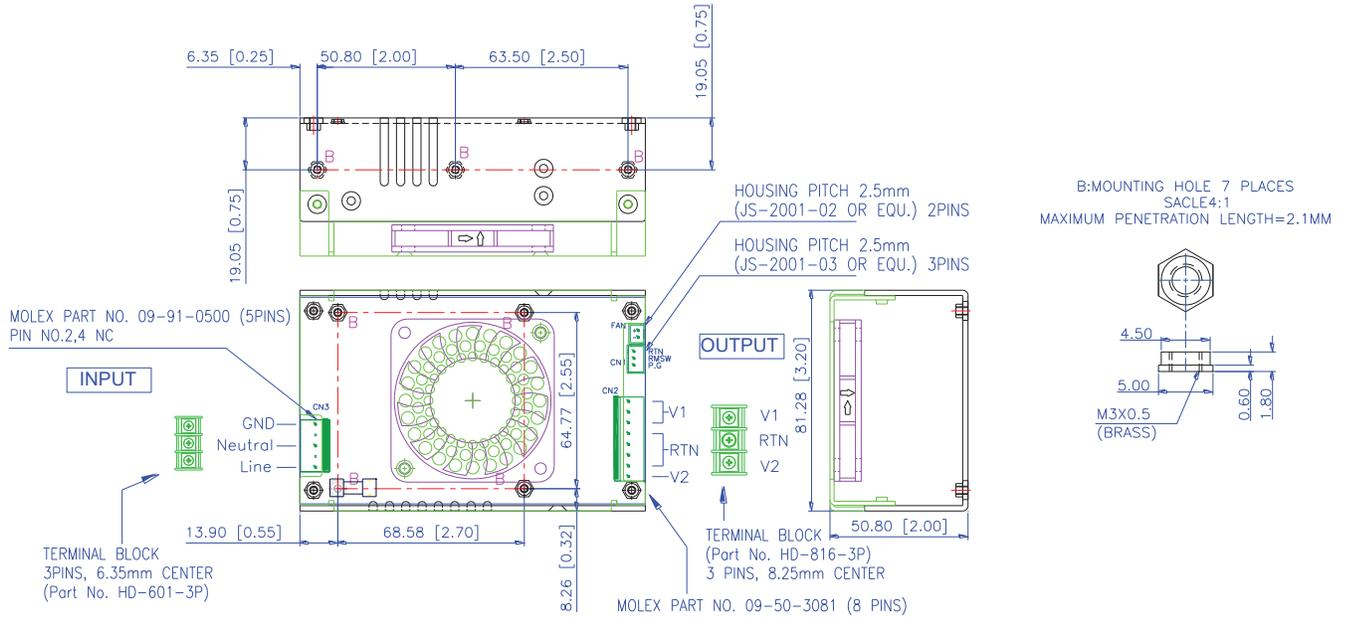
**RL0603DE Series (Enclosed with end built-in Fan): 5.39(L) x 3.2(W) x 1.6(H) inches; Weight: 550g.**
