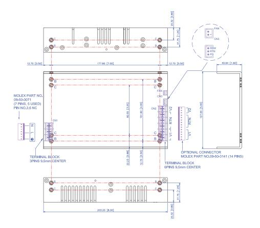
B: MOUNTING HOLE 8 PLACE 6-32 UNC(Zn-plated) SCALE 4:1
