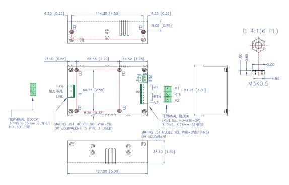
E Type (Enclosed with Rear Side built-in Fan): 6.5(L) x 3.2(W) x 1.6(H)inches; Weight: 650g.
