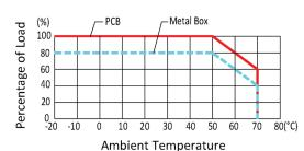
Note: Derate output power by 20% for enclosure (Metal Box) version.
