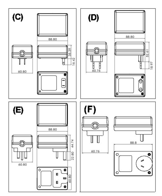
Suffix required to complete part # to define the mechanical package and output connector as illustrated in the mechanical drawings. For Example: AD1205y/xx (y = case/input plug configuration A-G | xx = 2.1, 2.5 or 1.3 (mm I.D. of output barrel plug). Default Polarity: Center positive, Add "N" to suffix for center (inner) connector negative. See Conncotro table or consult factory for additional connector options.
